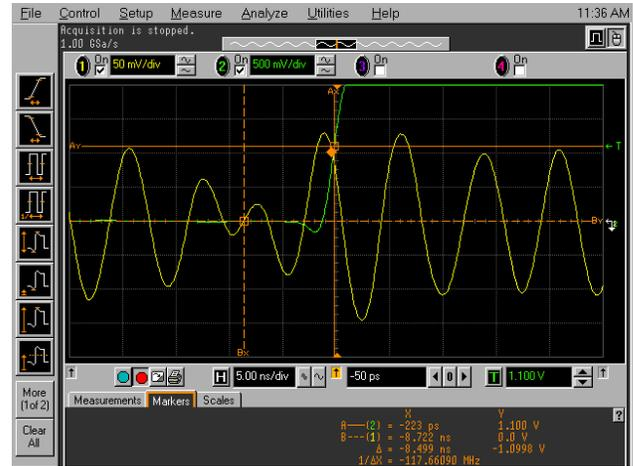
Figure 2—1PPS and IF on time point alignment
