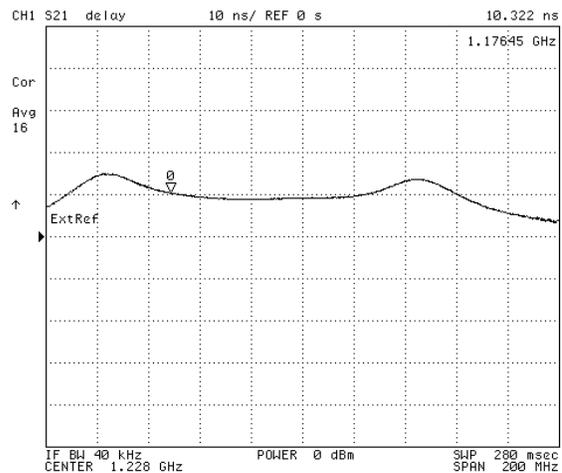
Figure 8- RF subsection group delay at 1176MHz (L5/E5/B2 band)
