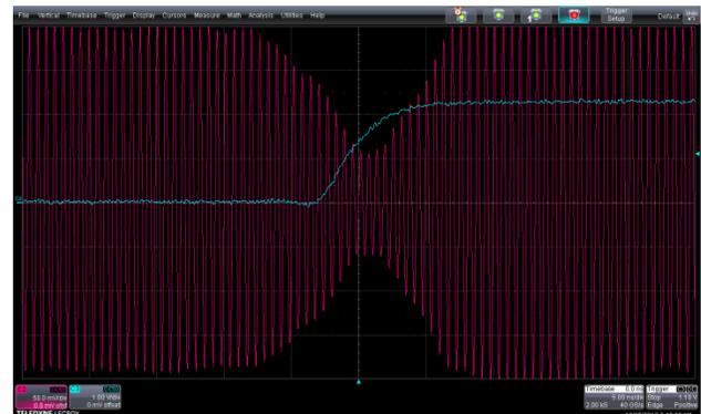
Figure 3—1PPS and RF on time point alignment
