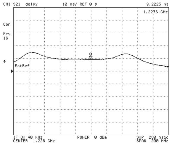
Figure 7- RF subsection group delay at 1228MHz (L2 band)
