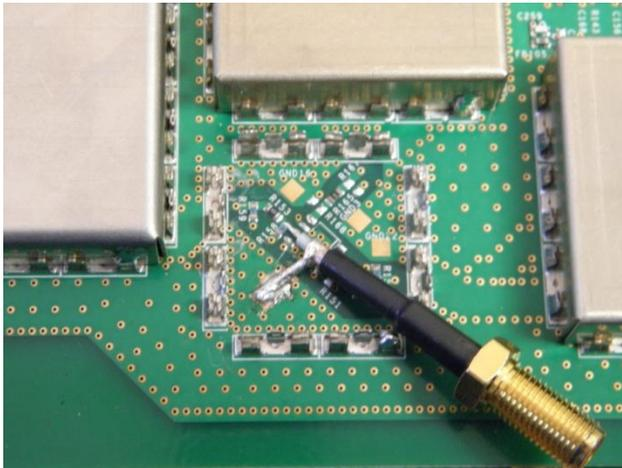
Figure 4—Mixer removal and replacement with SMA
