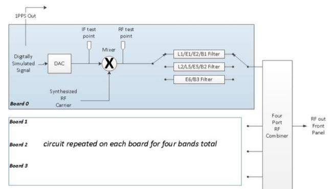
Figure 1 – Simulator Block Diagram
