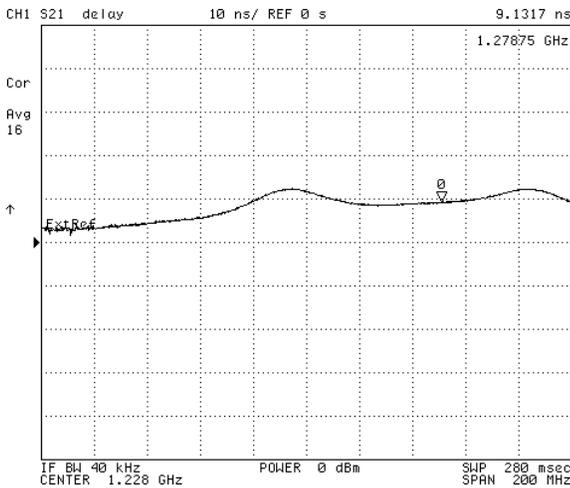
Figure 9- RF subsection group delay at 1279MHz (E6/B3 band)
