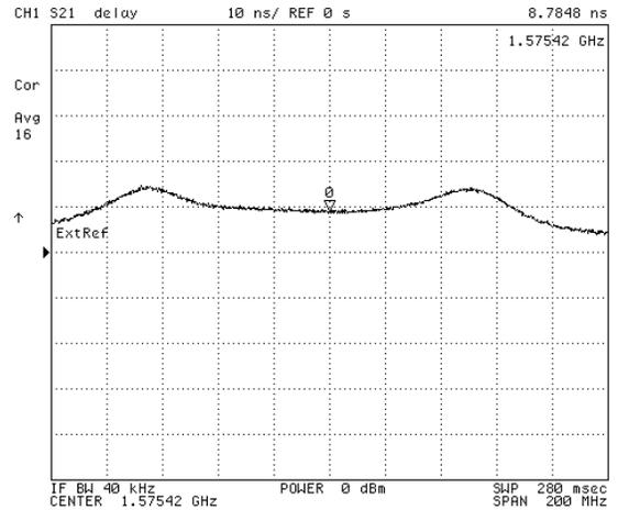
Figure 6- RF subsection group delay at 1575MHz (L1/E1/B1 band)
