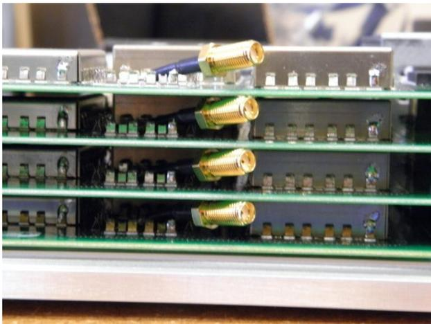
Figure 5—4 band GSG Simulator with SMAs installed
